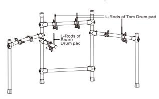
11. Assemble drum pads as shown.
