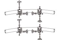
6. Connect the front pillar and side arm. Please confirm that the side arm is locked in the clamp of big joint.
