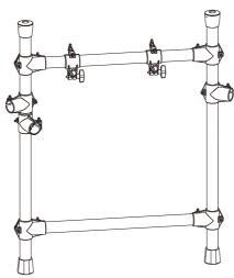
Note: When connect the back pillar and center pipe, please lock the center pipe in the clamp of the big joint to prevent the center pipe rotates.
